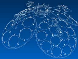
"LOPS" - Planetary for "Lift off" with 2 axis rotation
