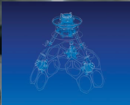
"Flip" planetary system for double sided coating
