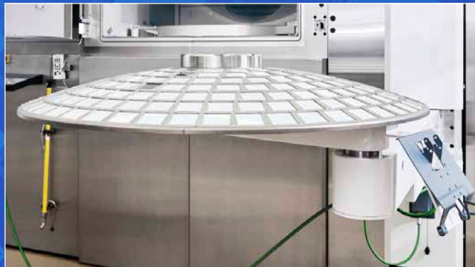
Large BAKs – option for calotte load / unload via robot
