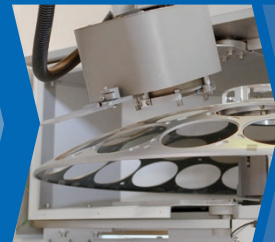
Dome loading including metrology wafers
